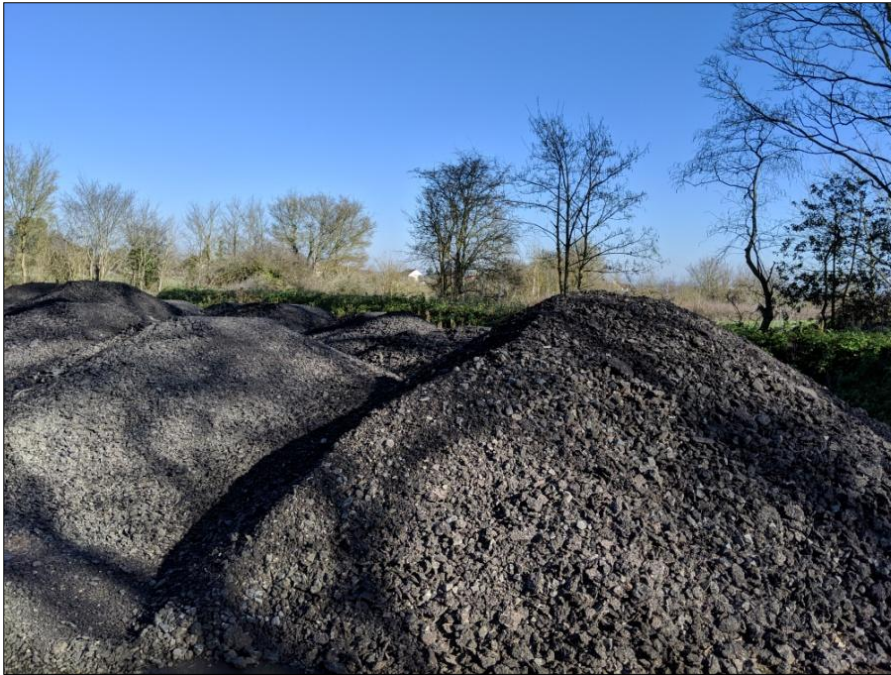
Road planings ready for reuse
